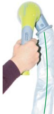
Withdraw the hose from the end of the bag. Using the hook and loop, thread the end of the hose over the exhaust up to the guard and wrap the hook and loop band tightly around the exhaust on the recess.
