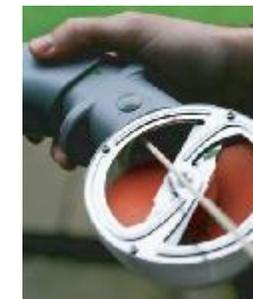
Switch off the machine, detach the hose, then detach the head from the main body of the machine (see page 8), with a long thin implement such as a stick, loosen the compacted material from the head or exhaust and empty into an appropriate receptacle, being careful to avoid touching the blade area with fingers. Once clear, re-attach head and hose to the machine, ensuring the growth you are attempting to cut is within the "fits and limits", the machine was originally designed for.
