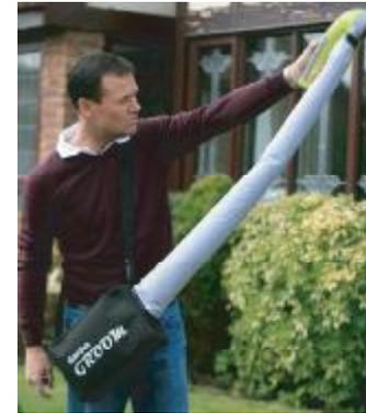
To reduce the build up of waste material in the hose, it is necessary to periodically pull the hose taut (as shown opposite) on an angle to allow the waste to flow freely into the bag. We also recommend this technique if there is a minor blockage in the head or exhaust of the machine, in order to create airflow and smooth conveyance of material.
